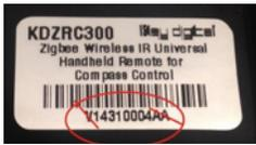
(Note: In the back of the remote, when removing the battery cover, there is a serial number on the bottom of a serial bar. The Device ID number is between the beginning and ending letters.)
